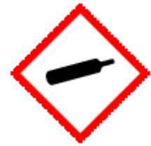
Ico 9.1.4 Gas under pressure
