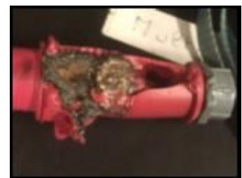
Pic. 7.4.6 Melted connector
