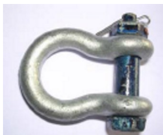
Pic. 10.2.13 Secured bolt anchor shackle
