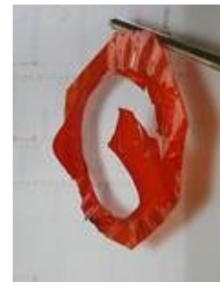
Pic. 5.7.3 Burned filter
