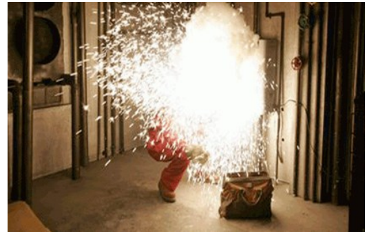
Pic. 7.2.2 Arc flash
