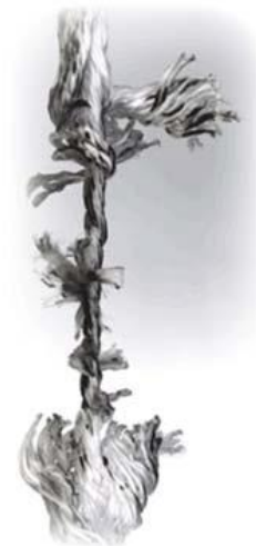
Pic. 10.2.36 Damaged rope
