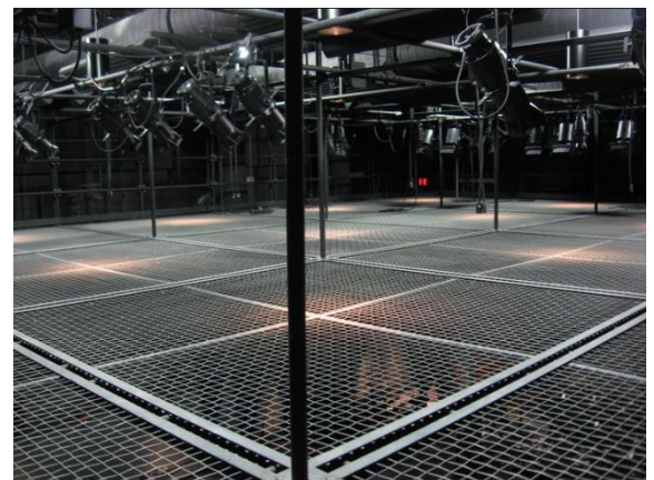
Pic. 10.3.3 Tension grid
