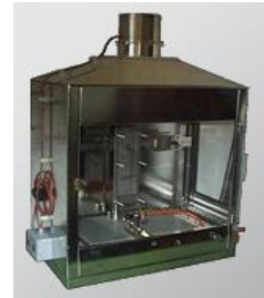
Pic. 5.7.2 Fire box
