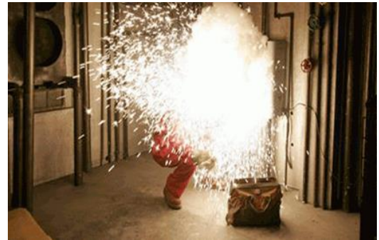
Pic. 7.2.2 Arc flash
