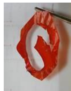
Pic. 5.7.3 Burned filter
