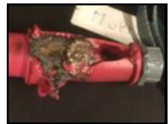
Pic. 7.4.6 Melted connector
