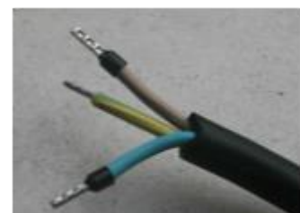
Pic. 7.4.1 ferrule on stranded wire
