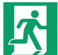
Ico. 5.6.2 Emergency exit right
