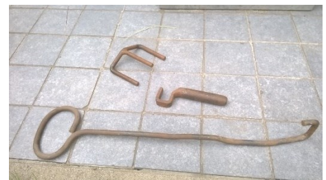
Foto. 3.3.20 Different types of scenery hooks, Ivo Kersmaekers
