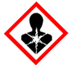
Ico 9.1.8 Serious health hazard
