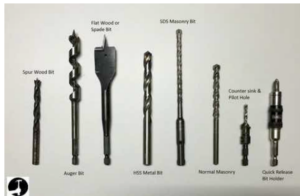
Pic. 8.0.1 different types of drills; verschiedene Arten von Bohrern
