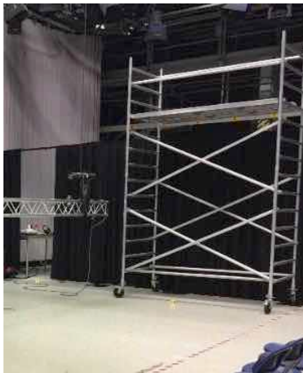
Pic. 6.0.3 mobile scaffolding
