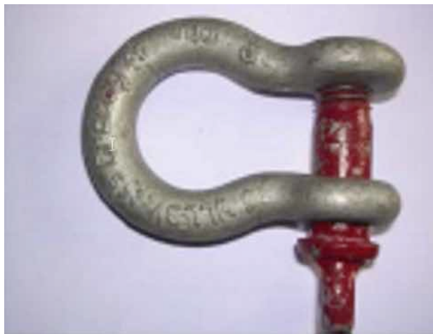
Pic. 10.2.14 Screw pin anchor shackle; Schraubbolzen-Ankerschäkel
